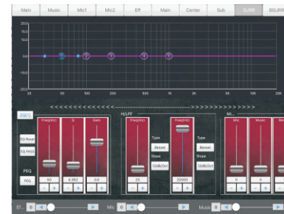
Surround output 5 bands PEQ+LPF/HPF+Mixer+Gain+ Delay+Limiter
